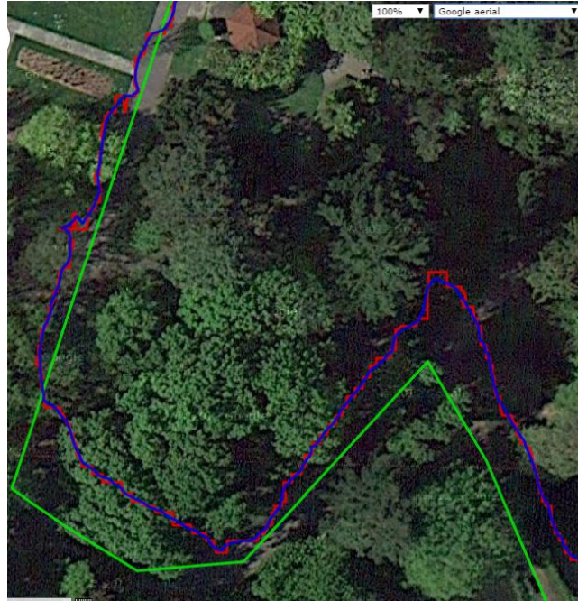
Fig. 4: Measurement 3 in Google Map. Red - measured data, blue - filtered data, green – road OSM data
