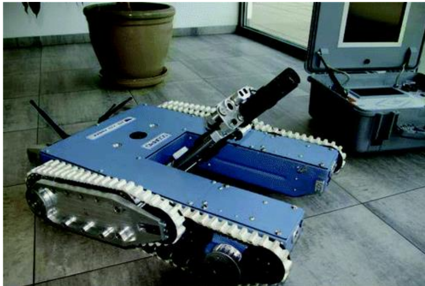
Fig. 2: Telerobot Scorpio - Ability of underpass the car, ability of explosive device disposal without the need of manipulation with it, possibility of remote control including the video transmission by radio signal, possibility of remote control including the video transmission through cable connection, simple control, obstacle avoidance and overpass, possibility of control and reconnaissance by visual systems, measuring of distance between obstacles and telerobotic system, detection of explosive device and measuring of distance between this device and muzzle of water gun and consequent disposal, possibility of simple implementation of additional extensions.
