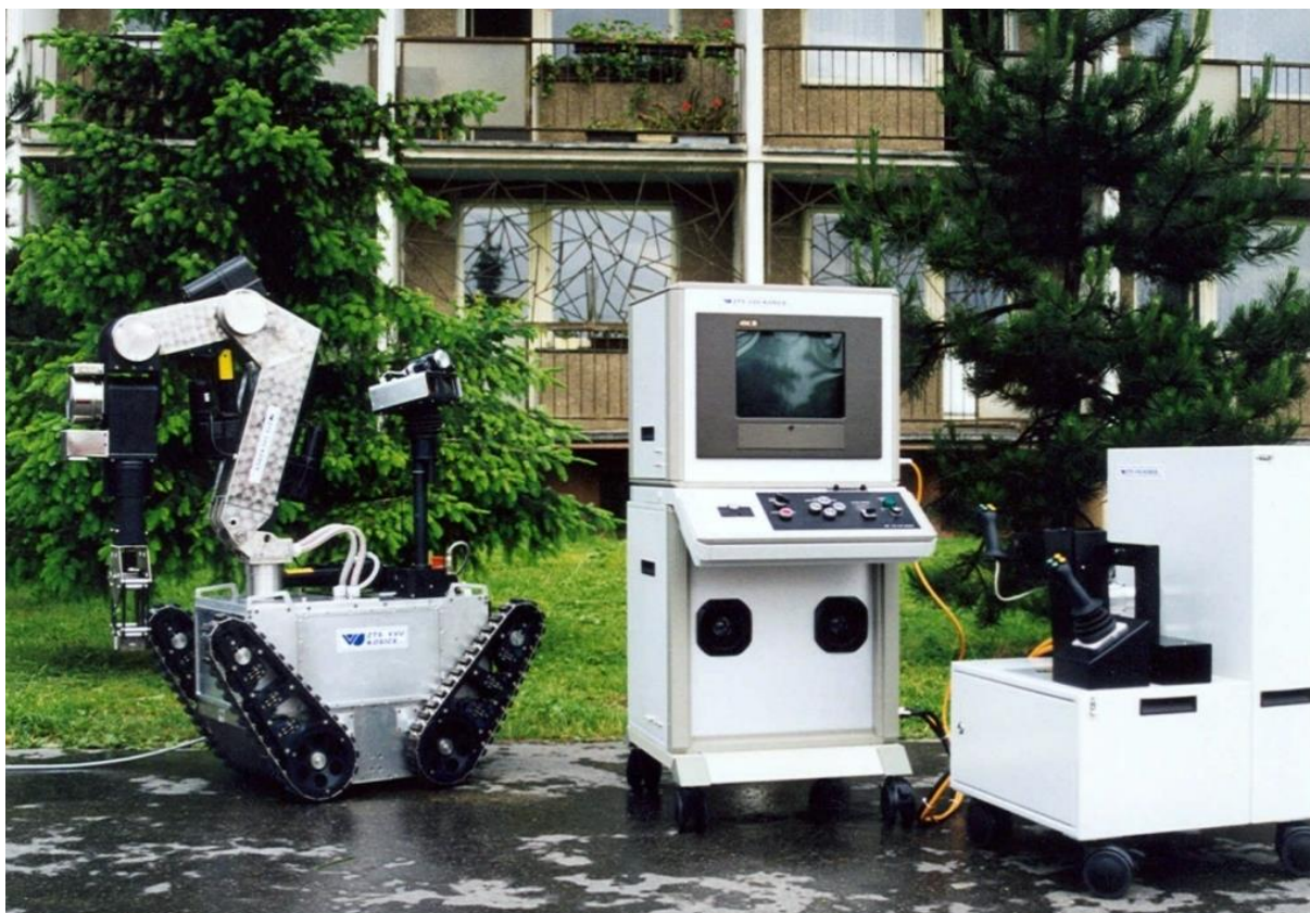
Fig. 4: Mobile manipulator MT-15KM - all movements are provided by electric motors. Main parameters: rotation + 45^\circ , main arm lift - 30^\circ to + 105^\circ , auxiliary arm lift + 105^\circ , wrist rotation \pm n \times 360^\circ , jaws opening max. 260 mm, weight 86 kg, payload - unloading 1,5 m - 15 kg, payload - unloading 0,5 m - 40 kg, installed power 475 W.
