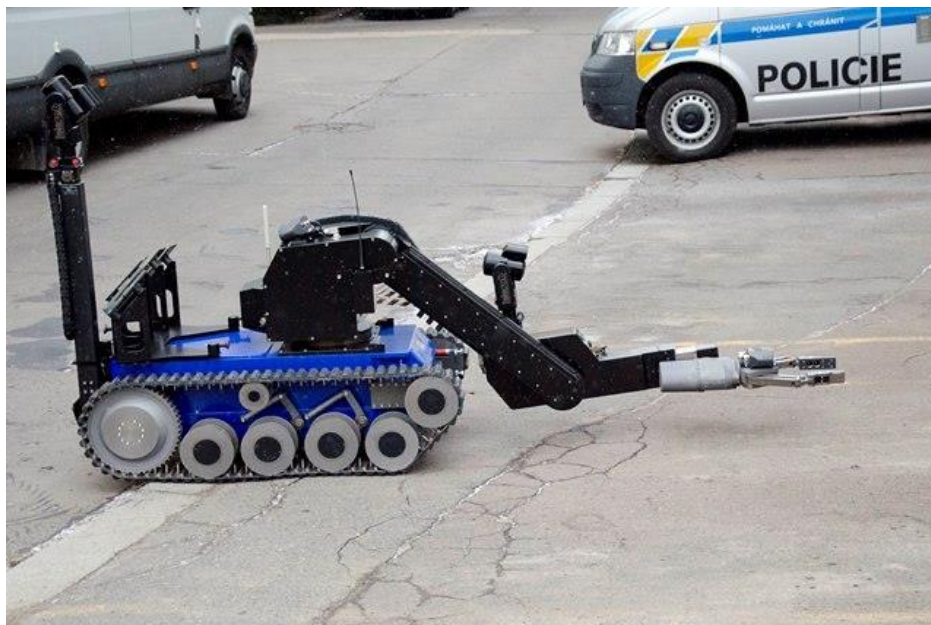
Fig. 3: Telerobot Teodor – main parameters: length 300 mm, width 685 mm, height 1 240 mm, weight 375 kg, speed max. 3 km/h, payload 350 kg, operation time 3-4 hours. Control station: weight 86 kg. Control panel: weight 9 kg.
