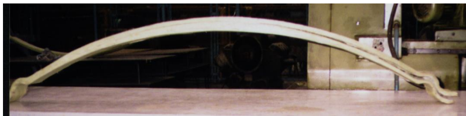
Fig.6. Example of damaged composite spring
