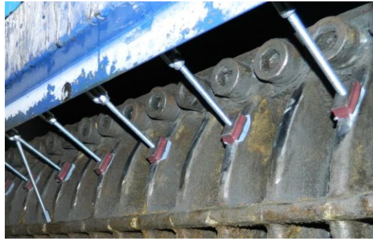
Fig. 4: Applying of the pressure during the adhesive curing
