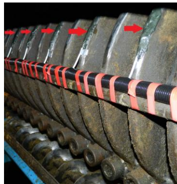
Fig. 5: Final measured ribs of the basket with protected strain gauges and wiring
