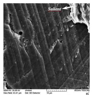
Fig. 8: Intercrystalline facet, right side of the sample
