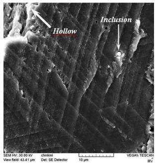
Fig. 9: Intercrystalline facet, left side of the sample
