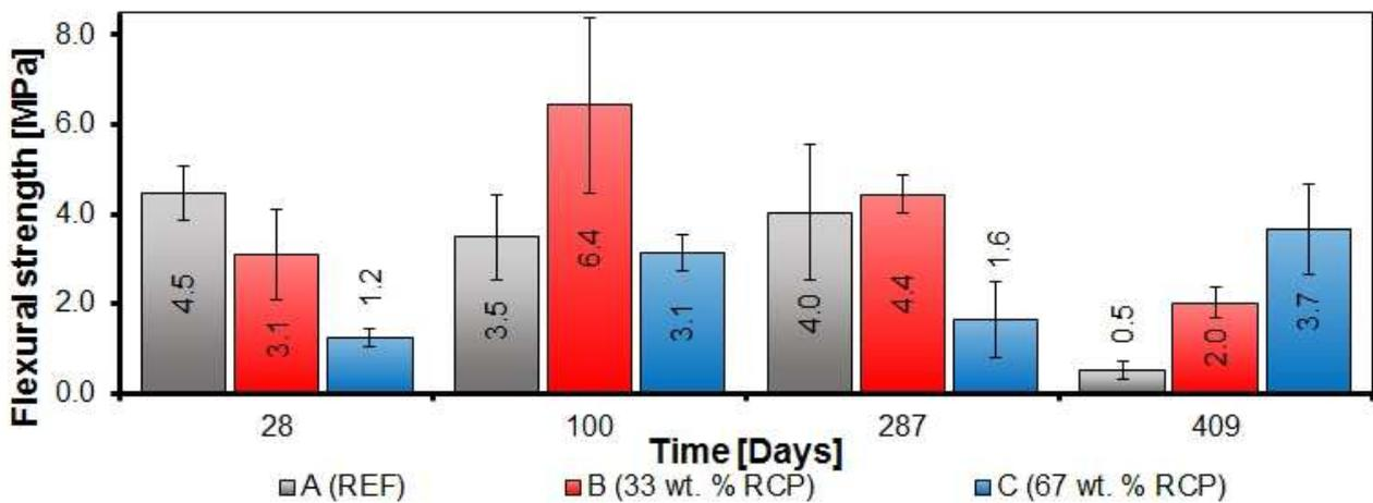
Fig. 1: Flexural strength development of the cement pastes with different amount of a recycled concrete powder.
