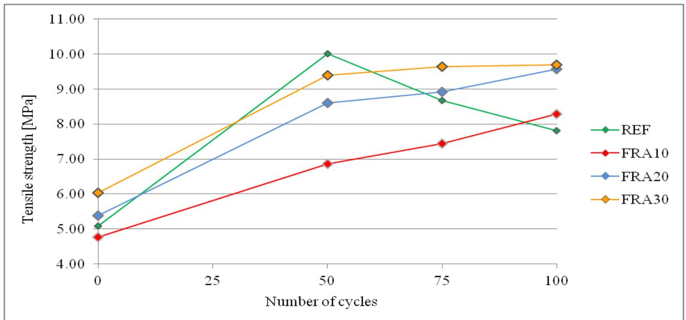
Fig. 3: Test results of tensile strength after 50, 75 and 100 freeze – thaw cycles
