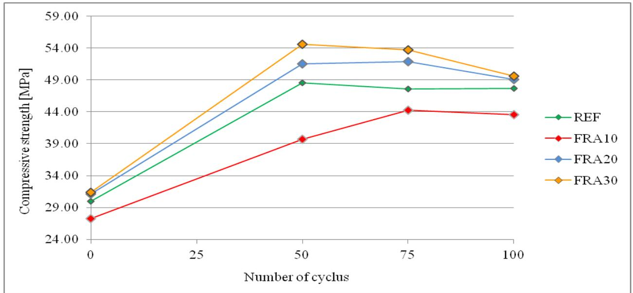
Fig. 2: Test results of compressive strength after 50, 75 and 100 freeze – thaw cycles
