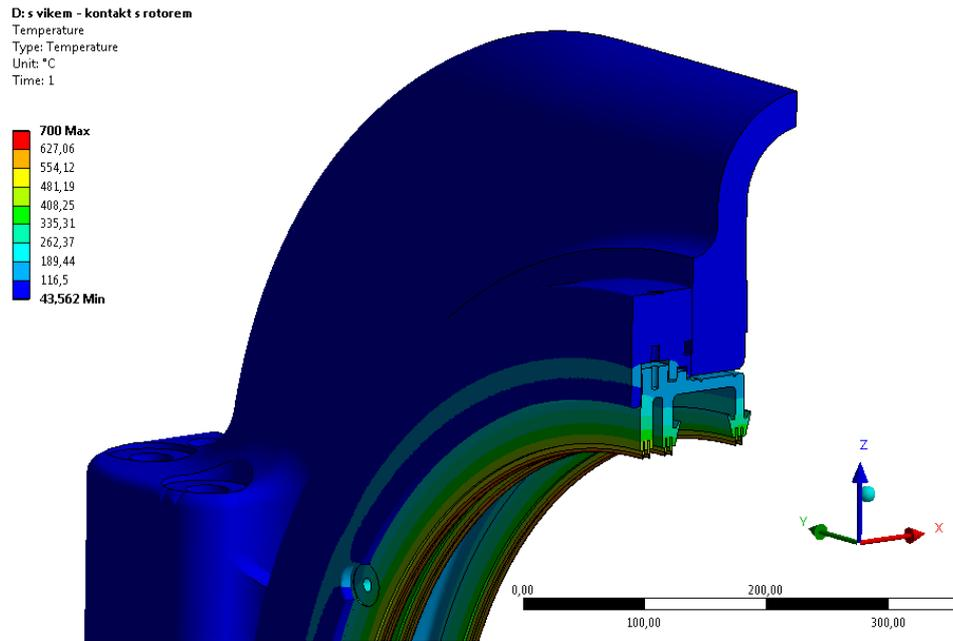
Fig. 1: Temperature field of the assembly
