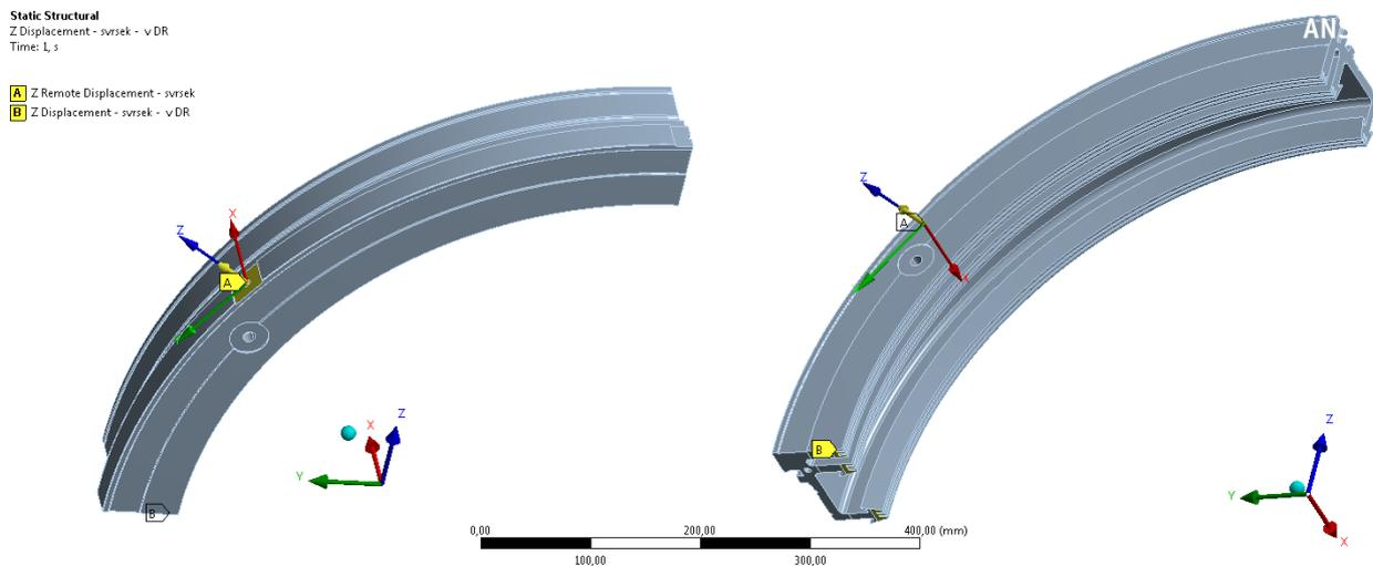
Fig. 4: Boundary condition - displacement
