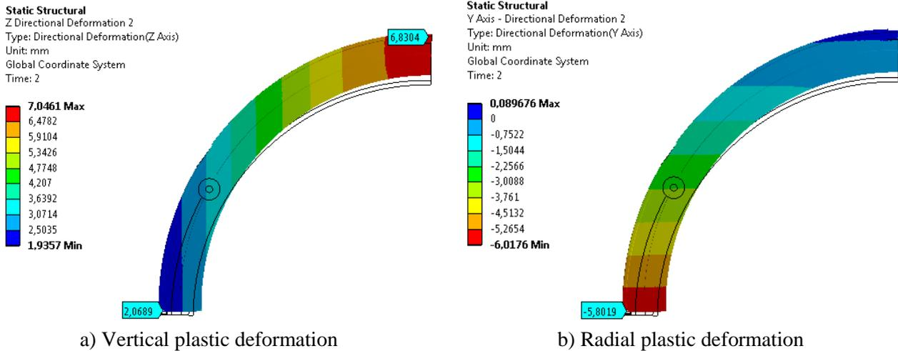
Fig. 5: Final shape after elastic-plastic deformation
