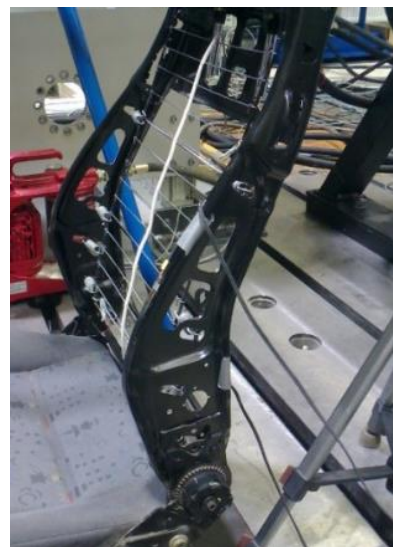
Fig. 4: Loading of the backrest (defined by a force or an equivalent torque) and position the strain gauges
