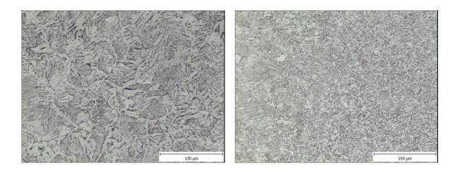
Fig. 1 The microstructure in weld metal
