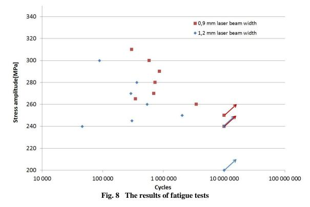
Two specimens were prepared and tested from other sheets/shielding gases. All specimens were tested at the same stress amplitude -255MPa - slightly above fatigue limit. The results of this comparison are summarized in Table 4. The values from sheets with argon shielding gas were statistically calculated from Wöhler curves of each sheet.
