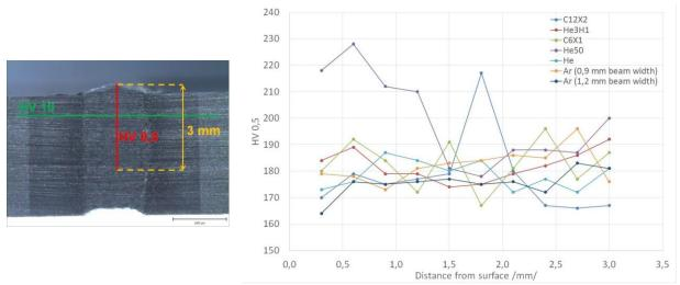
Fig. 5 and 6 Summary of microhardness HV0,5 profile measurement
