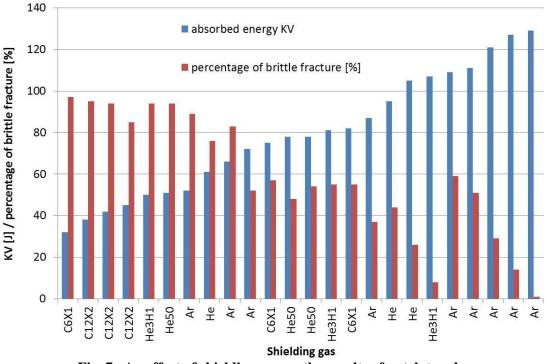
Fig. 7 An effect of shielding gas on the results of notch toughness
