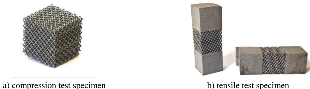
Fig. 1: Trabecular structure specimens for global mechanical tests.
