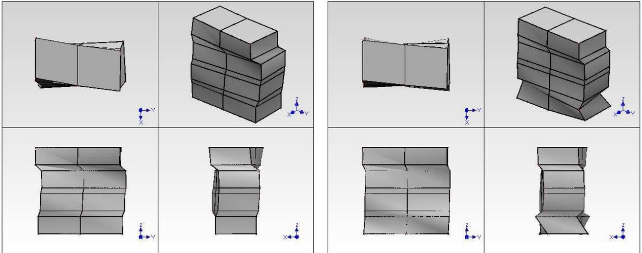
Fig. 3: The 1<sup>st</sup> natural mode of vibration of the specimen LMK\_S\_2,  $f_1 = 1153$  Hz
