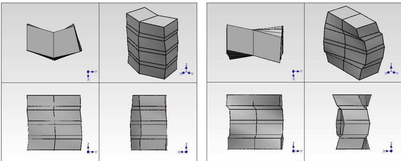
Fig. 2: The 3<sup>rd</sup> and 4<sup>th</sup> natural modes of the specimen LMK\_SCB\_2,  $f_3 = 3027$  Hz and  $f_4 = 3247$  Hz
