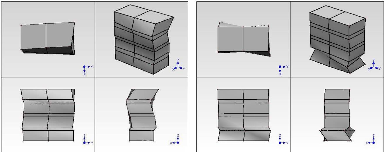
Fig. 4: The 2<sup>nd</sup> natural mode of vibration of the specimen LMK\_S\_2,  $f_2 = 1497$  Hz
