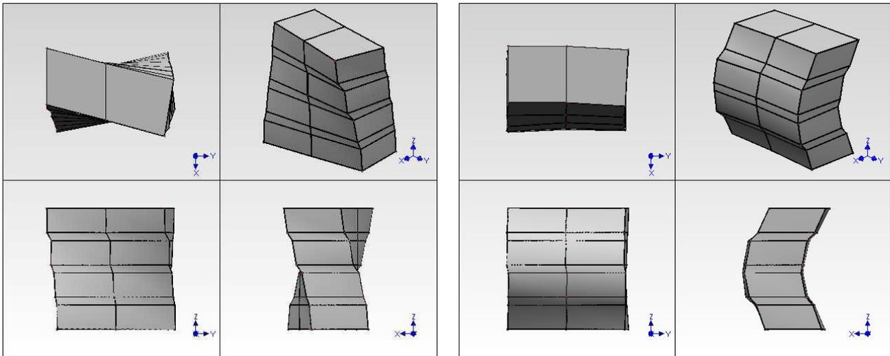
Fig. 1: The 1<sup>st</sup> and 2<sup>nd</sup> natural modes of the specimen LMK\_SCB\_2,  $f_1 = 1715$  Hz and  $f_2 = 2298$  Hz
