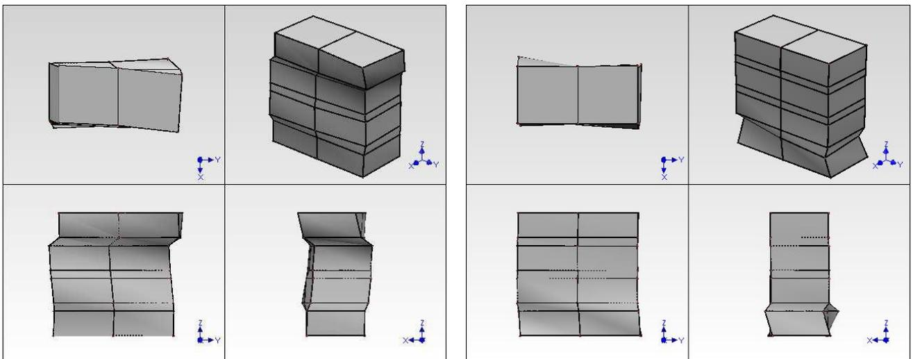
Fig. 5: The 3<sup>rd</sup> natural mode of vibration of the specimen LMK\_S\_2,  $f_3 = 1735$  Hz
