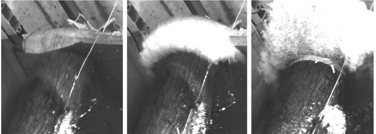
Fig. 4: Time response of detail impact of wood log on the plate of flood barrier
