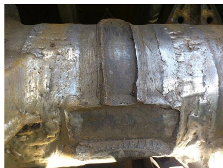
Fig. 9: Fractured surface on the shaft of the rotor
