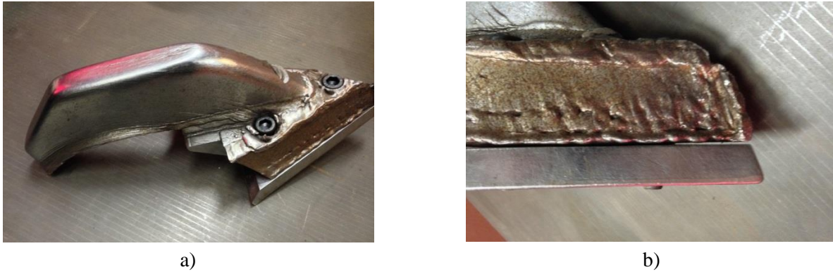
Fig. 6: Knife holder with a moving knife- fixed by three bolts a) top view, b) side view.
