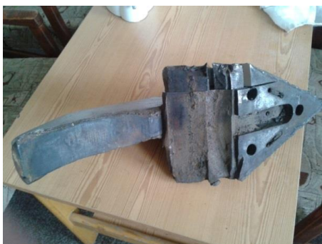
Fig. 8: Broken holder with moving knife
