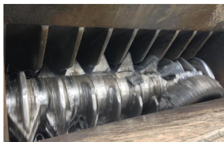
Fig. 3: Tyre shredding crushing in the shredding machine
