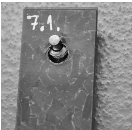
Fig. 6: Right failure mode for bearing stress evaluation.
