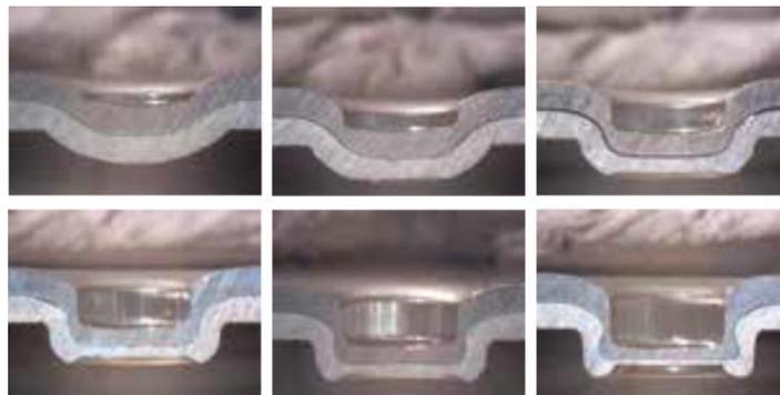
Fig. 1: TOX®-Round Joint formation, [1]
