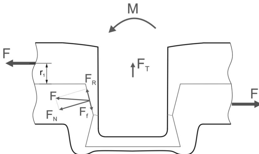
Fig. 4: Computational scheme of the joint
