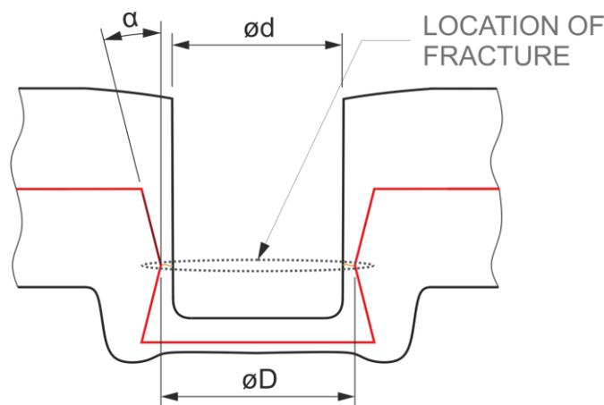
Fig. 4: Simplified scheme of the joint
