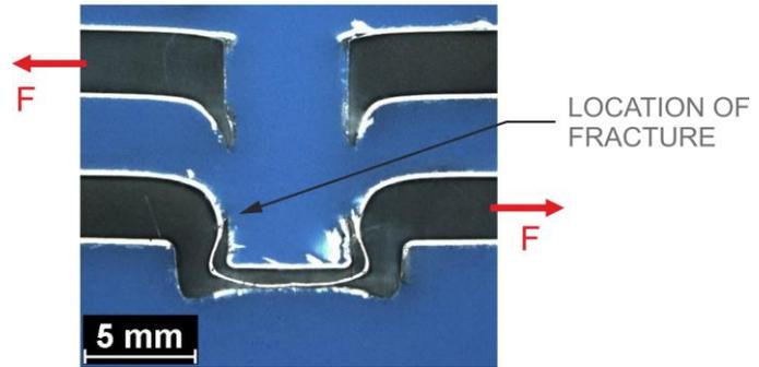
Fig. 3: Clinched joint – fracture after the single lap shear test in the joint neck
