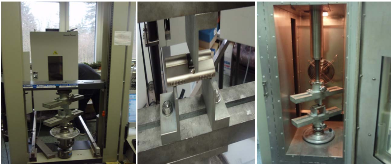
Fig. 1: Testing of cylindrical locks outside and inside the thermal chamber.
