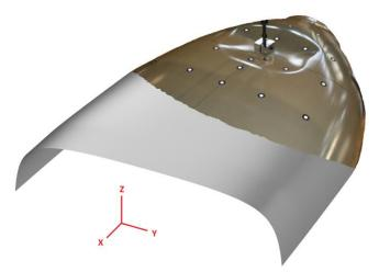
Fig. 9: Deformation shape of nacelle during test
