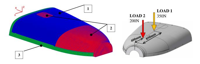
Fig. 3: Positions of monolithic laminate and sandwich composite
