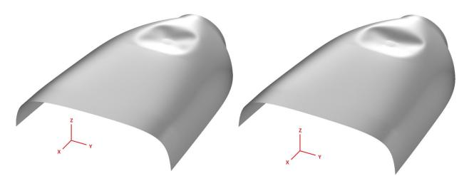
Fig. 7: Nacelle with constrained all 6 degrees of Fig. 8: Deformation shape of nacelle with gap freedom on free edges elements on free edges
