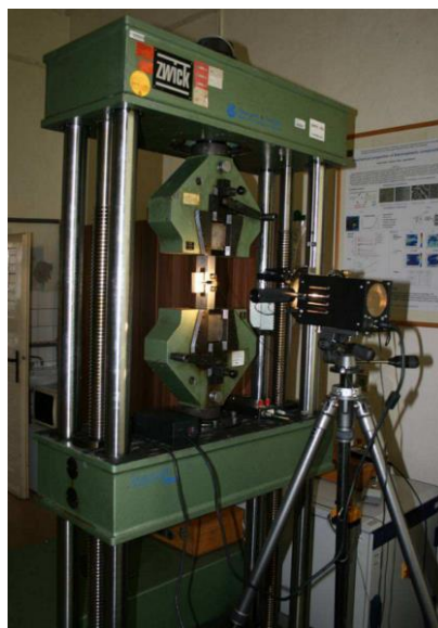
Fig. 3: Tearing machine Zwick 1387 and reflection polariscope LF/Z-2.
