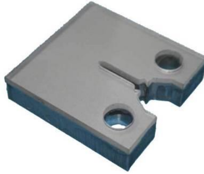
Fig. 2: Analyzed sample with photoelastic coating.
