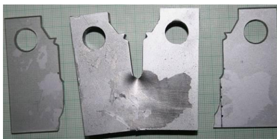
Fig. 14: Damaged photoelastic coating PS-1A with the notched sample and relative elongation 4%.
