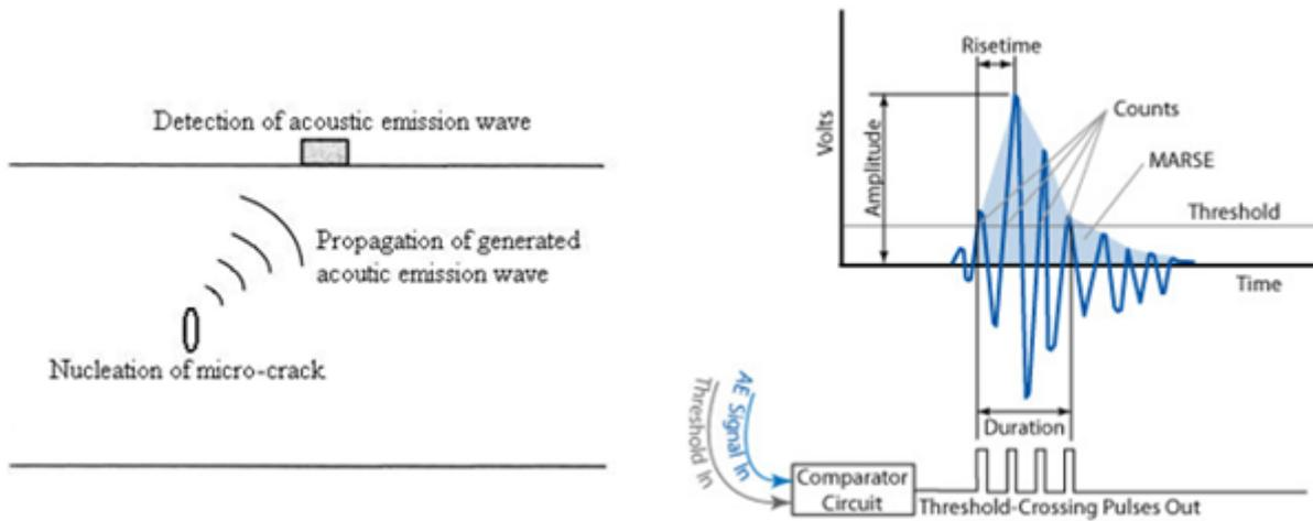
Fig. 1: Detection of AE wave [7] and typically AE signal [8].
