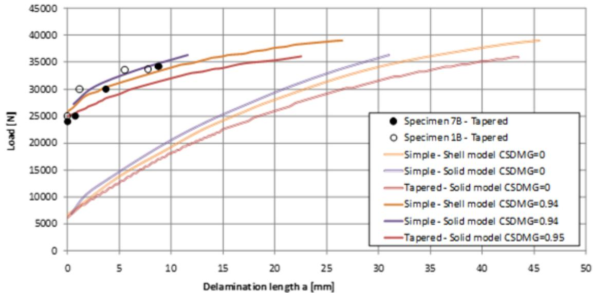
Fig. 4: Delamination growth; tapered and simple lap bond joint FE models, experiment.
