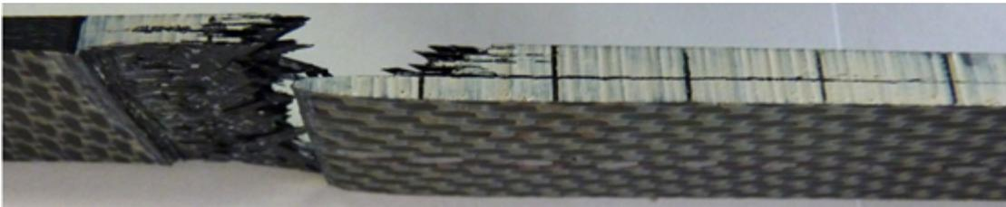
Fig. 2: Typical fracture of the tension specimen.
