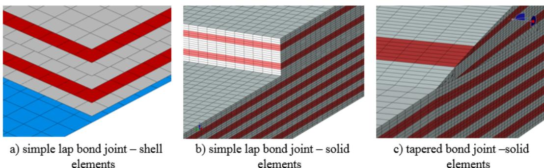
Fig. 3: FE models of tension specimens – detail.
