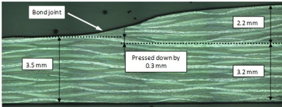
Fig. 1: Detail image of layer stacking in the vicinity of the bond joint.
