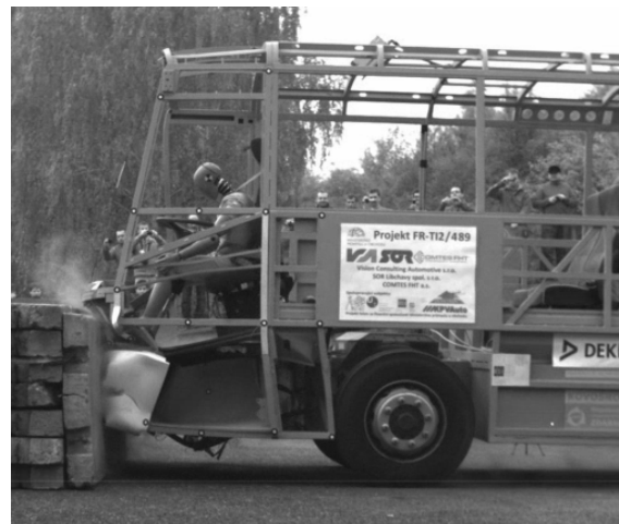
Fig. 14: Full-Scale Frontal Crash Test.
