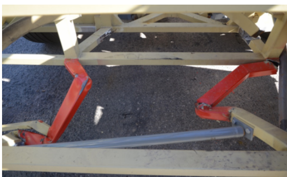
Fig. 17: Chassis Deformed after the Crash.
