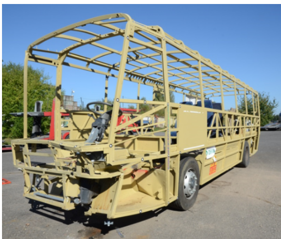
Fig. 15: Vehicle after Frontal Crash.
