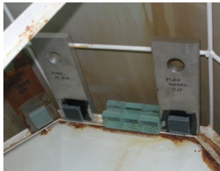
Fig. 4: Testing setup for glass-to-metal specimens.
