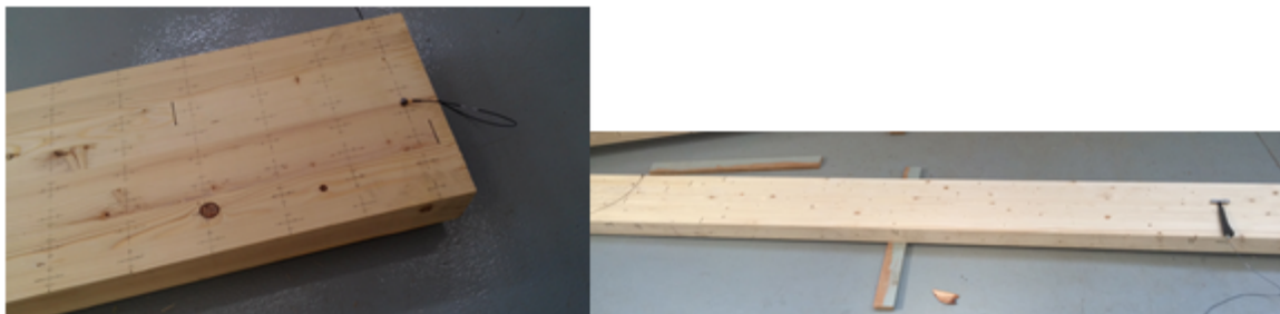
Fig. 2: Setting up the sensor and driver for flexural natural frequencies s measurement.
