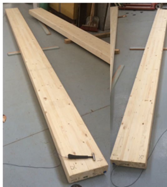
Fig. 3: Setting up the sensor and driver for longitudinal natural frequencies measurement.
