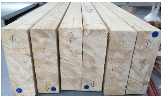
Fig. 1: Second set of Glued laminated timber beams.
