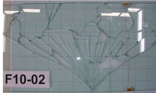
Fig. 3: Typical failure mode of test specimens.
