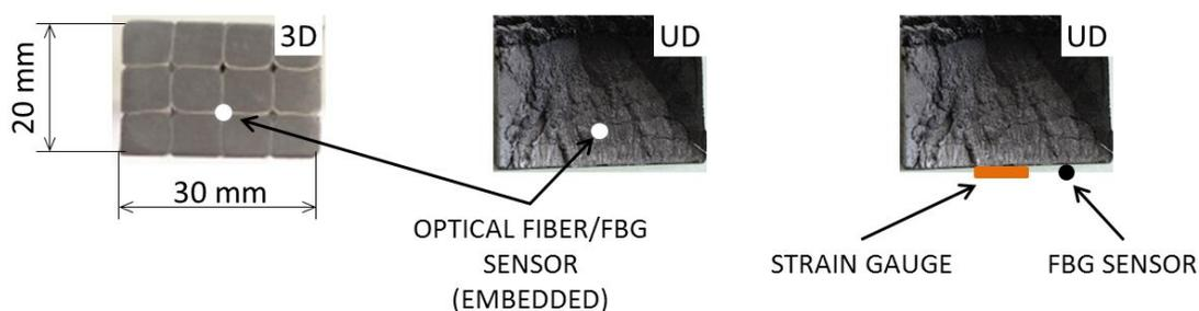
Fig. 1: Cross sections of specimens with locations of strain sensors.
