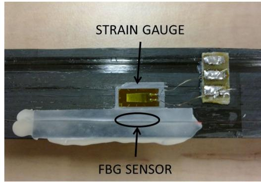
Fig. 2: Location of surface-mounted strain sensors.
