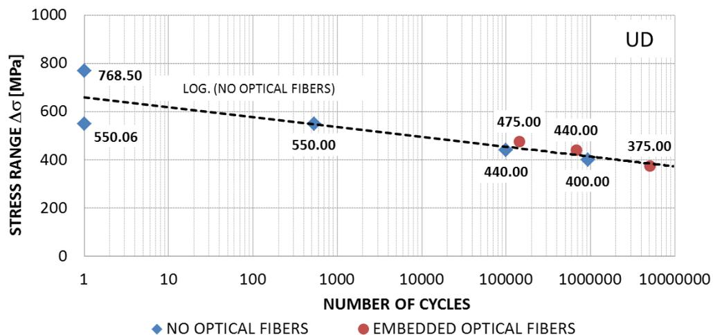
Fig. 4: Fatigue S-N curve for UD Carbon/Epoxy specimens.
