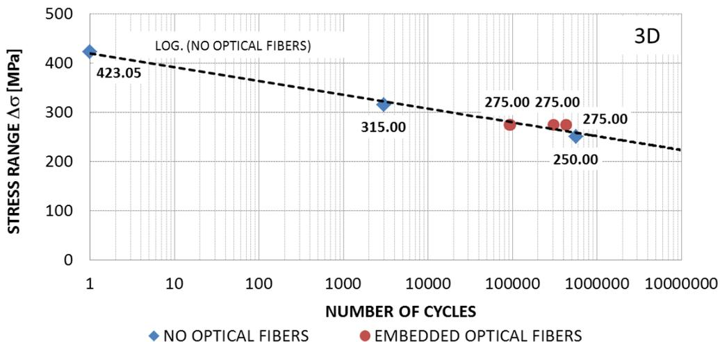
Fig. 5: Fatigue S-N curve for 3D Carbon/Epoxy specimens.
