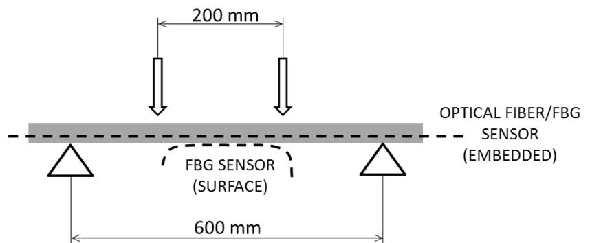
(b) specimen and sensors configuration
