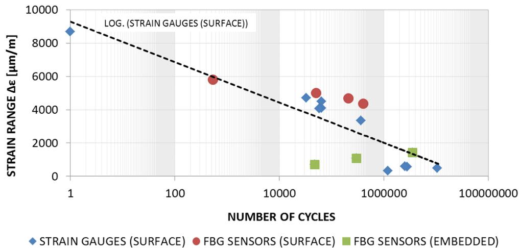
Fig. 6: Fatigue S-N curve for Carbon/Epoxy specimens with surface-mounted strain sensors.
