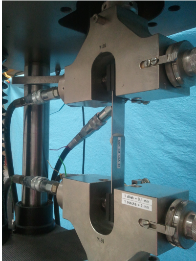
Fig. 1: Adhesive joint specimen during shear test.
