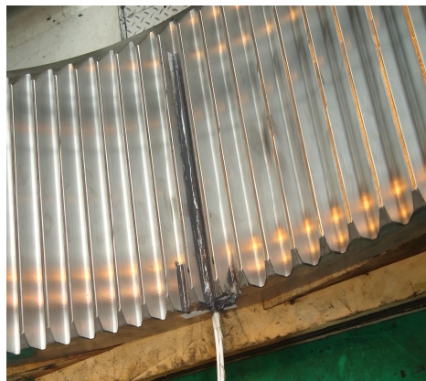
Fig. 4. Strain gauges on ring gear (with epoxide layer).
