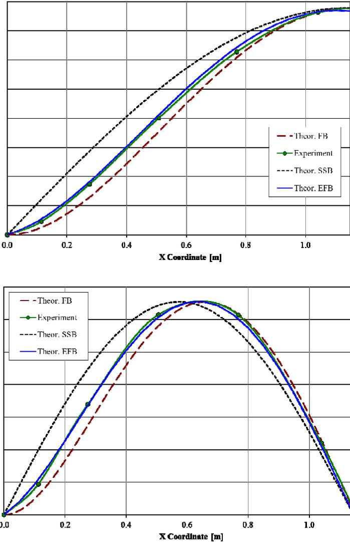
Fig. 3. The steel rod No. 1c – the comparison of the theoretical and measured natural mode shapes on the half of the rod length (above – the 1<sup>st</sup> mode shapes, below – the 2<sup>nd</sup> mode shapes).
