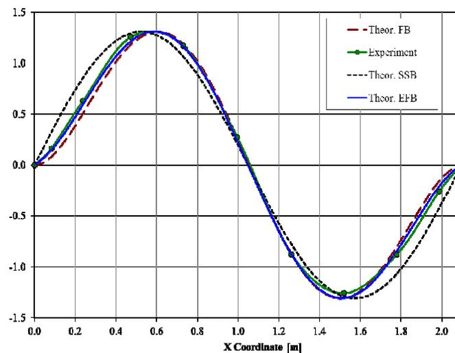
Fig. 2. The steel rod No. 1a – the comparison of the theoretical and measured 2<sup>nd</sup> natural mode shapes.
