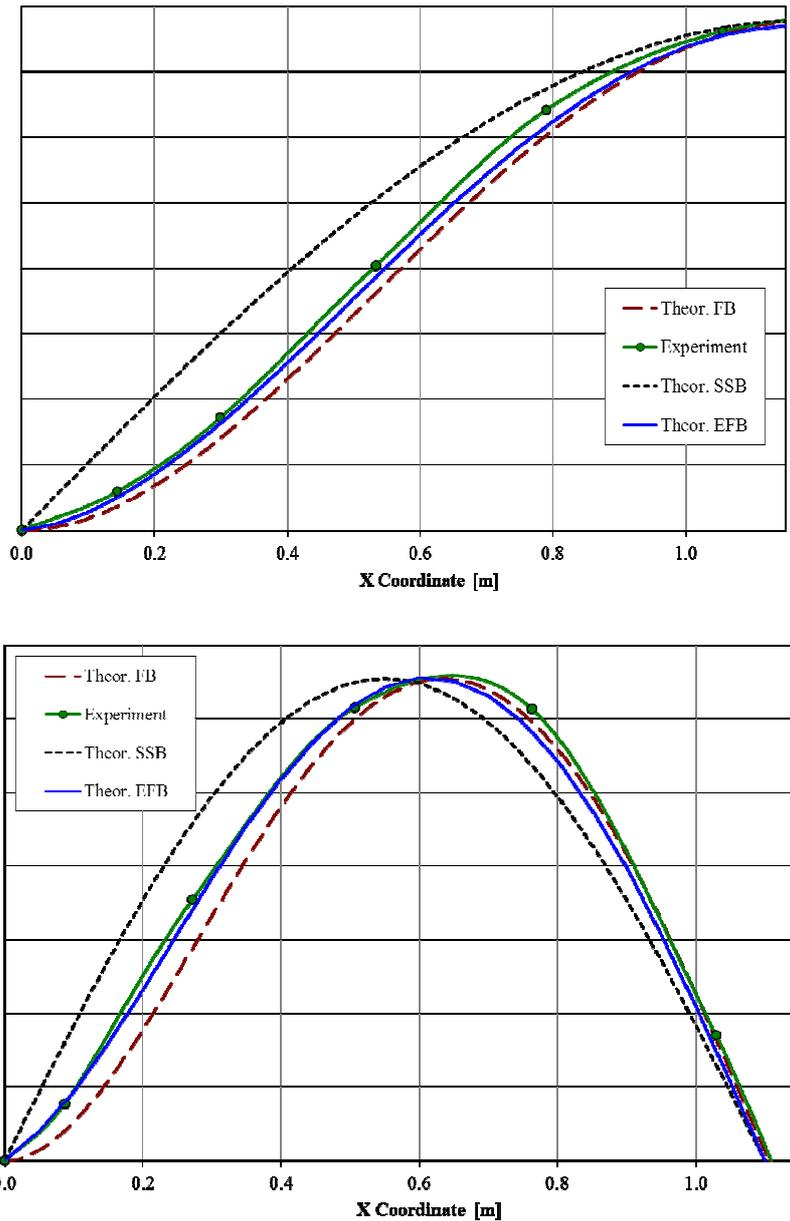
Fig. 4. The comparison of the theoretical and measured natural mode shapes (above – the 1<sup>st</sup> mode shapes of the steel rod No. 2d, below – the 2<sup>nd</sup> mode shapes of the steel rod No. 3b).
