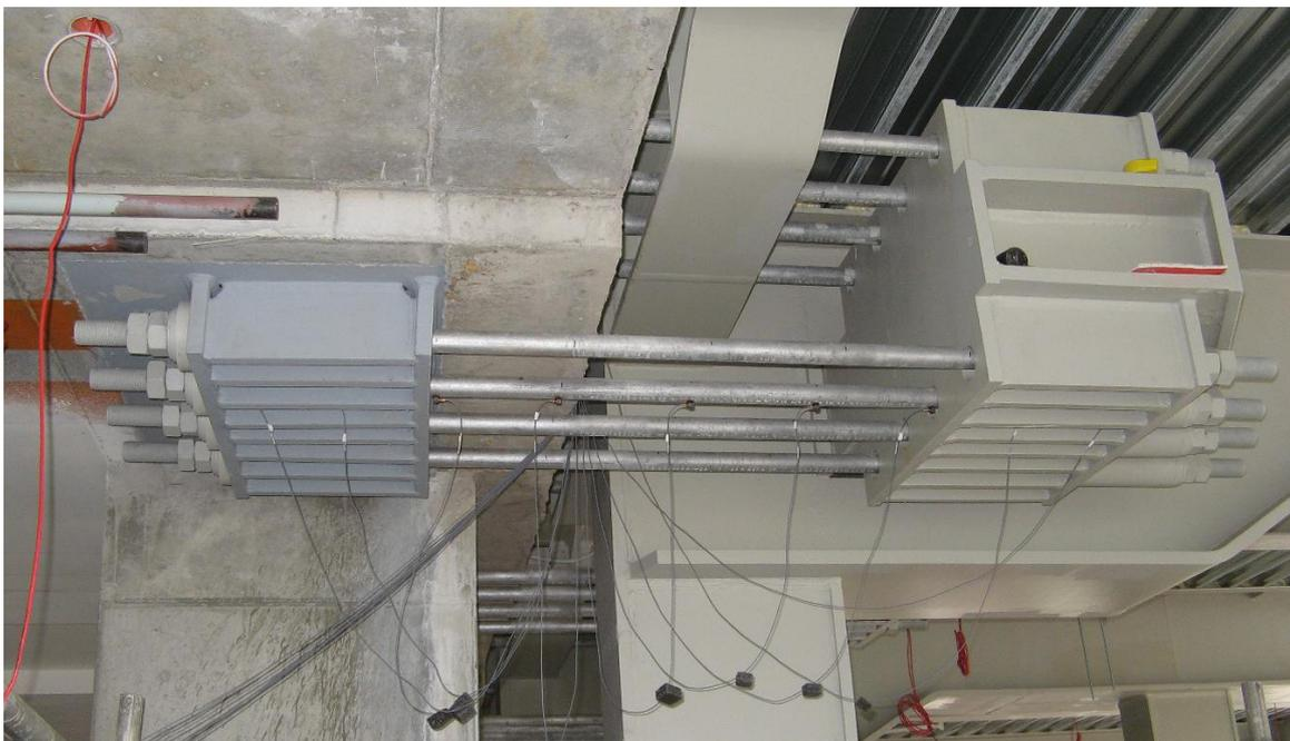
Fig. 1. The view on the four investigated steel rods (the rods No. 1a, 1b, 1c and 1d) and on the placed accelerometers on the rod No. 1b.
