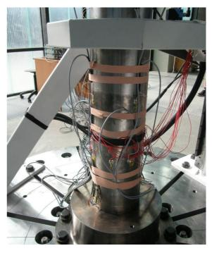
Fig. 2. Axle with all strain gauges at different disrance from hub.
