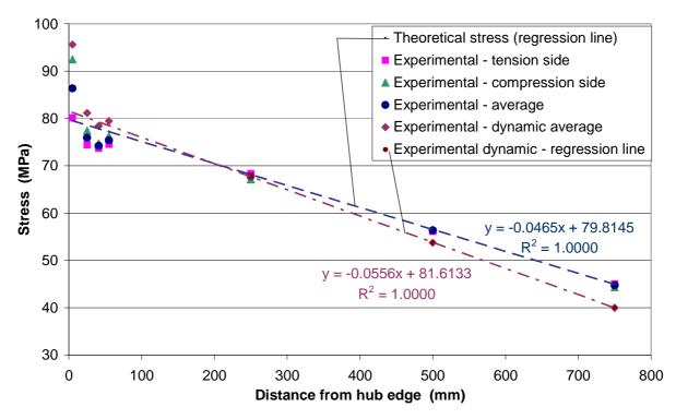
Fig. 3. Experimentally evaluated stress values on the axle surface during static and dynamic bending in comparison with theoretical values.
