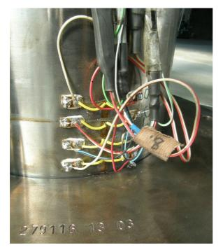
Fig. 1. Chain of strain gagues near hub edge.
