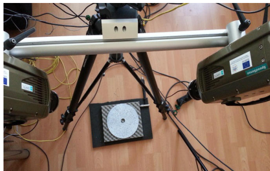
Fig. 3. Process of saw blade measuring with using of digital image correlation method.
