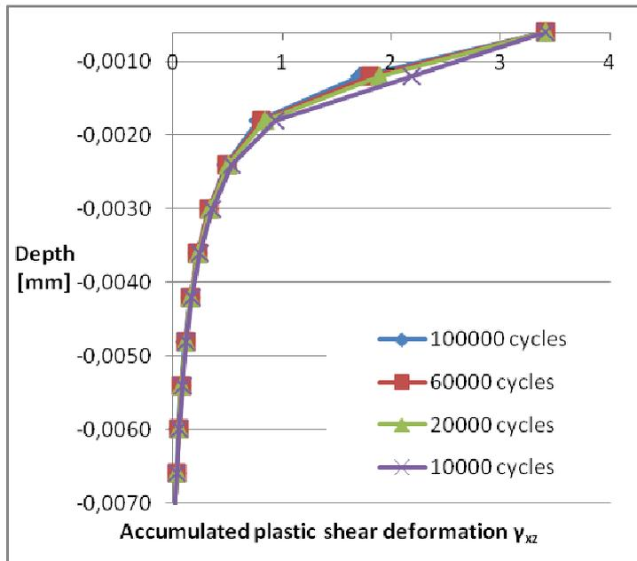
Fig. 7. Accumulated plastic shear strain profiles.
