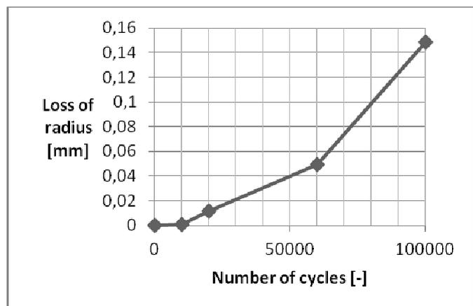
Fig. 3. Worn depth as the function of number of cycles.
