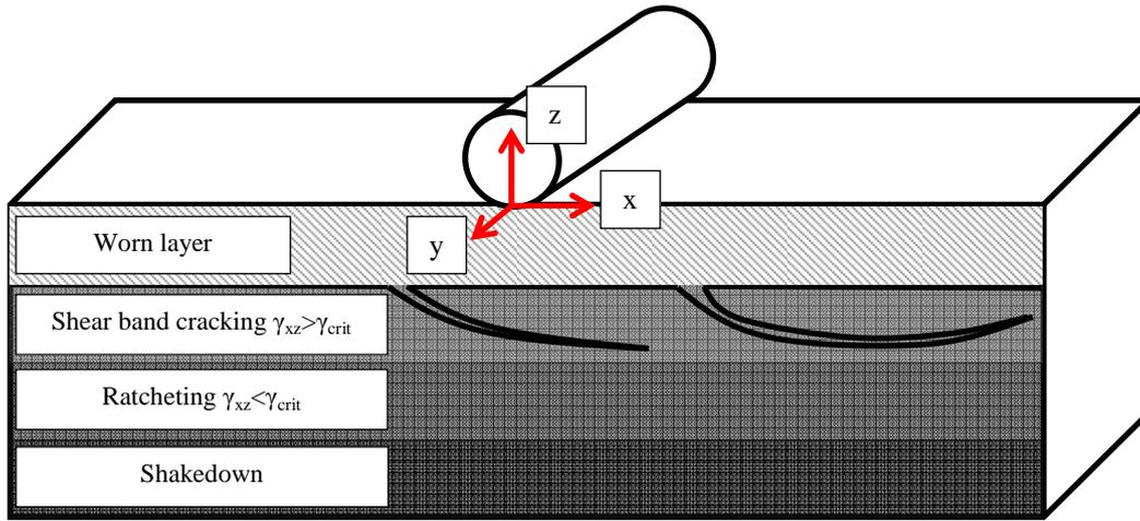
Fig. 6. Shear band cracking mechanism.
