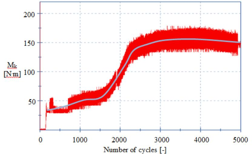
Fig. 4. Torque record for the first 5000 cycles.
