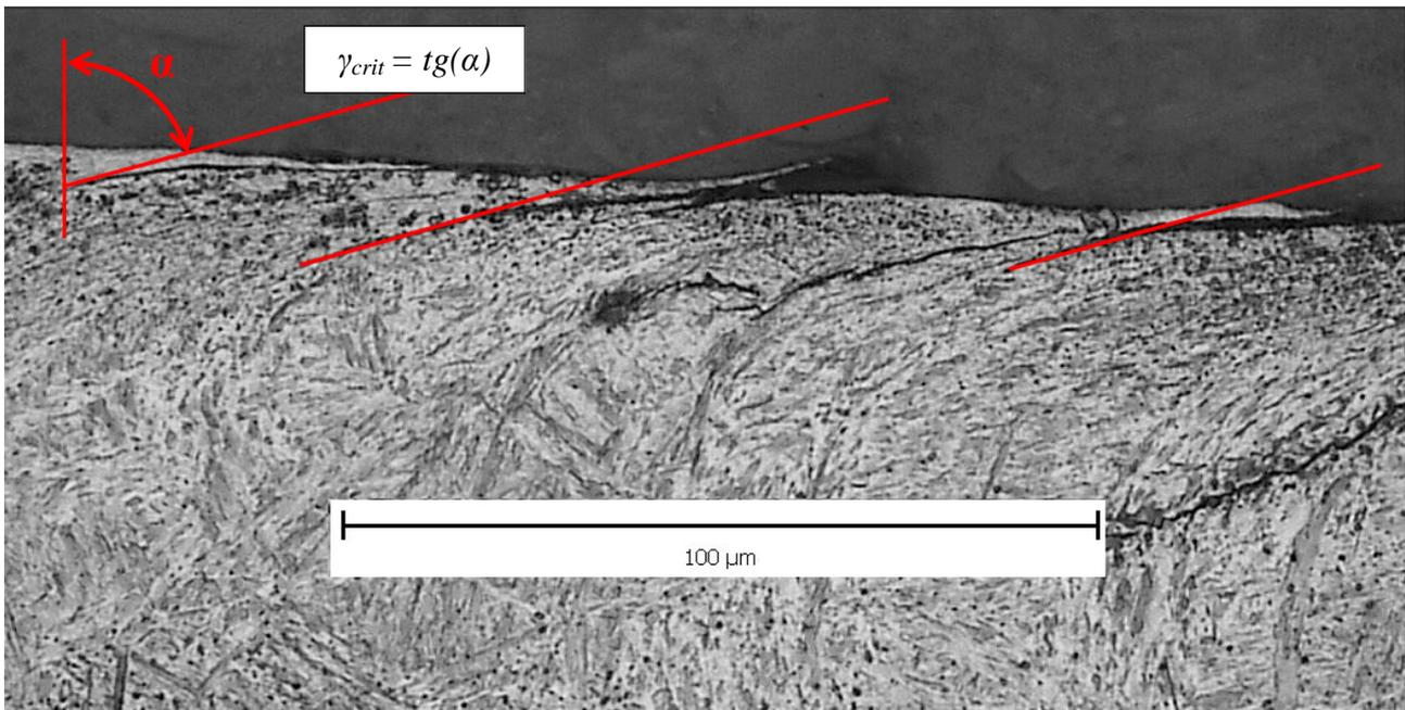
Fig. 5. Evaluation of critical plastic shear deformation.
