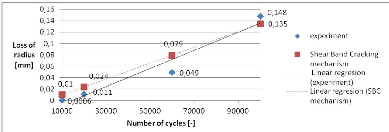
Fig. 9. Loss of radius as the function of number of cycles.
