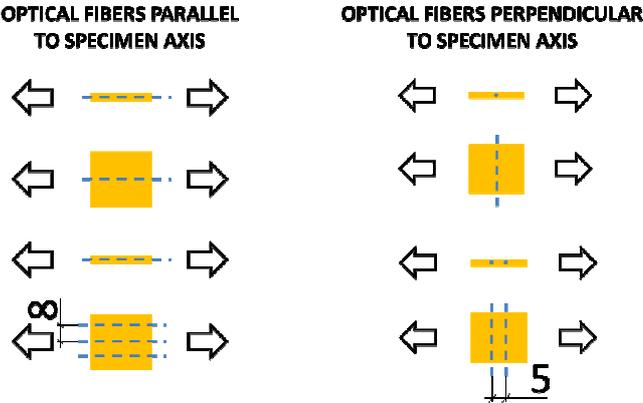
Fig. 2. Configurations of fibers in an adhesive layer.
