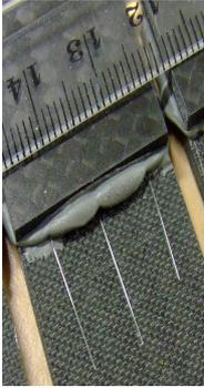
Fig. 3. Detail of optical fibers in an adhesive joint (conf. C).
