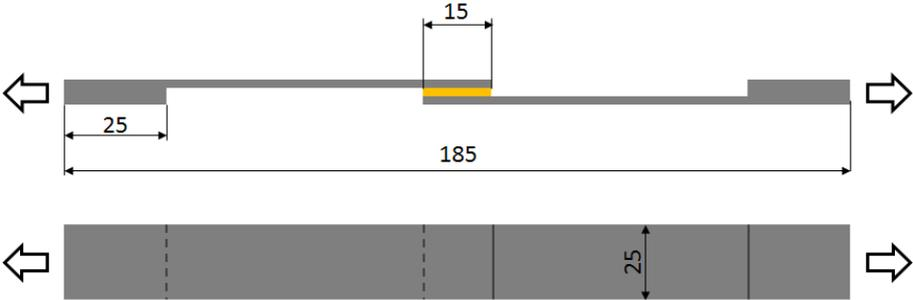
Fig. 1. Configuration and dimensions of tested specimen.
