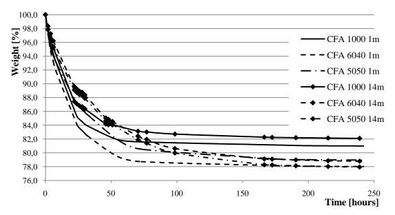
Fig. 1: Percentage change in weight of specimens of cement paste with different proportion of fly ash in time due to drying
