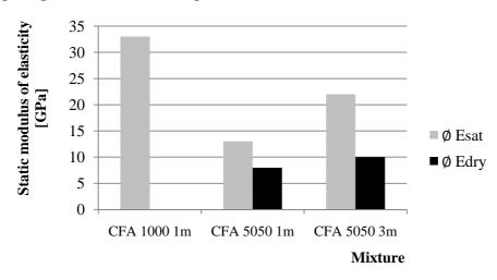
Fig. 3: The average values of static modulus of elasticity for each mixture and time
