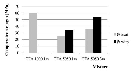
Fig. 2: The average values of compressive strength for each mixture and time
