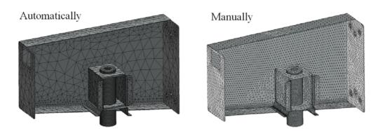
Fig. 4 – Automatically and manually generated mesh
