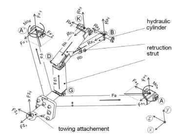
Fig. 2 – Application forces and reactions on trailer hitch
