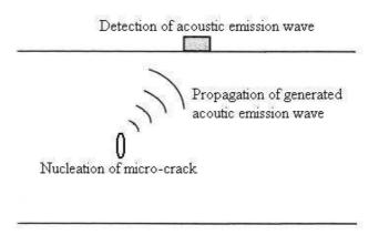
Figure 1: Detection of acoustic emission wave [8]
