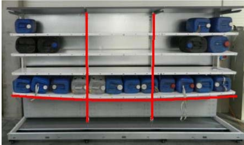
Fig. 6, Loading and deformation of the rack during testing
