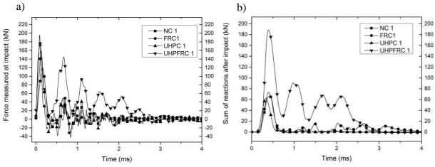
Figure 4. History of forces measured at the a) hammer tup and at the b) supports in first 4 ms after impact.
