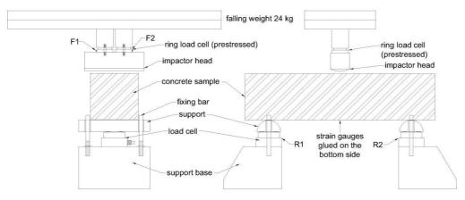
Figure 2: Sample position and instrumentation of the supports and impactor.
