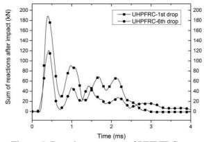
Figure 5. Reaction response of UHPFRC specimen, comparison between  $1^{st}$  and  $6^{th}$  hit.
