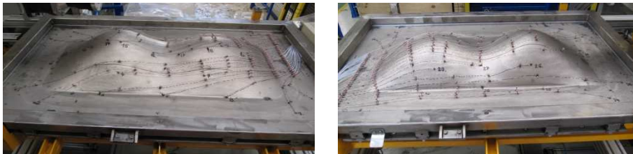
Fig. 2. Experimental galvanomould with defined geometric shapes
