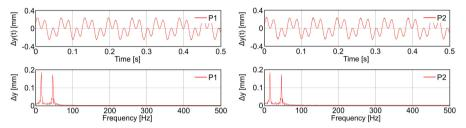
Fig. 12. Time and frequency dependence of automobile cooling fan vibration amplitudes in y direction determined in points P1 and P2
