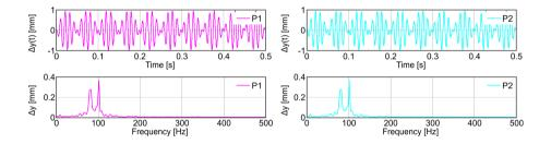
Fig. 6. Time and frequency dependence of oscillation displacement of cooling fan model of points P1 and P2 in y direction
