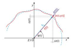
Fig. 1. Estimation of vibration amplitudes of a rotating object
