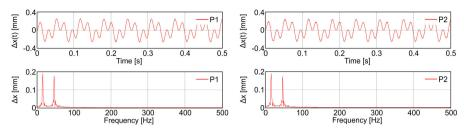
Fig. 11. Time and frequency dependence of automobile cooling fan vibration amplitudes in x direction determined in points P1 and P2
