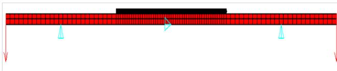
**Fig. 5: 4-point bending load configuration.**
