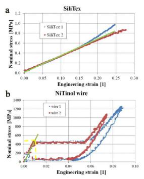
**Fig. 3.** (a) - Uniaxial loading of the silicon-textile matrix.  $E_M$  was determined as the initial slope of the tangent of the loading curve (green line). (b) - Uniaxial loading of NiTinol wire.  $E_W$  was determined as the initial slope of the tangent of the loading curve (green line). The transformation state ( $\sigma_{TW}$ ) is defined at the start of the plateau (yellow dashed line).
