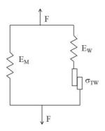
Fig. 2. Parallel elastoplastic rheological model of the homogenized composite. Left arm represents the elastic silicon-textile matrix while right arm refers to the ideal plastic NiTinol wire.
