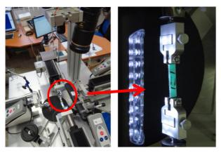
Fig. 1. On the left-Messphysic biaxial testing machine (Zwick/Roell). On the right- detail of the clamped sample.
