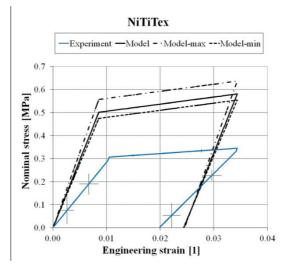
**Fig. 4.** – Uniaxial loading of the NiTiTex composite. The experimental curve (blue curve) is evaluated as the average of two measurements. Error bars include both measurements error and inter-sample variance. Model curve is evaluated for the medium, maximum and minimum cross-section.
