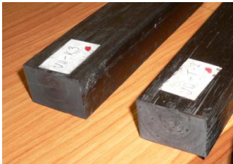
Fig. 1. Cross-section of thick-walled UD carbon composite specimens.
