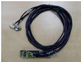
Fig. 3. Specimen made of unidirectional Carbon/Epoxy composite (Dialead k63712).
