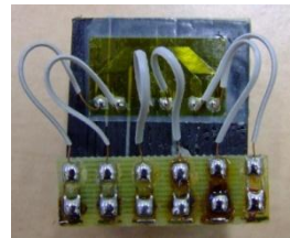
Fig. 4. Detail of HBM 1-RY81-6/350 strain gage rosette installation.
