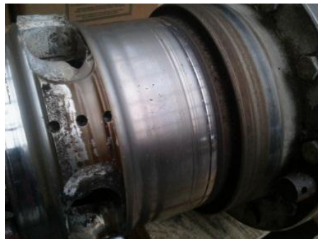
Fig. 1. Example of worn part of decanter centrifuge housing made of austenitic steel after 30 000 working hours (4000 rev./min).
