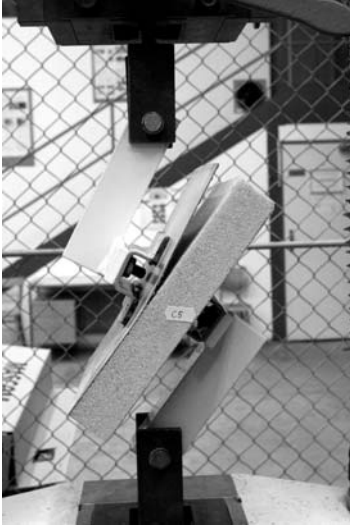
Fig. 3. Tensile testing of girder bracket
