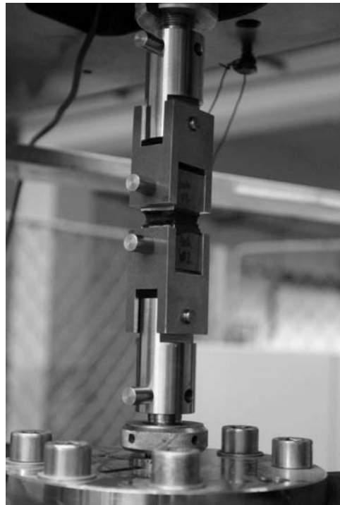
Fig. 2. Setup of tension test of adhesive
