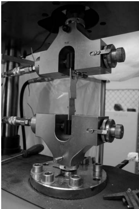
Fig. 1. Setup of shear test of adhesive
