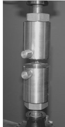
Fig. 3. Workplace for fatigue testing on small test specimens and the miniature test specimens grips (taken from [2])
