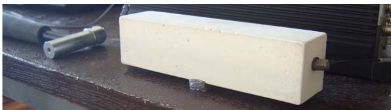
Fig. 1. The impulse excitation method – test arrangement for measurement of fundamental longitudinal resonant frequency
