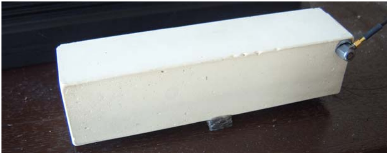
Fig. 3. The impulse excitation method – test arrangement for measurement of fundamental torsional resonant frequency
