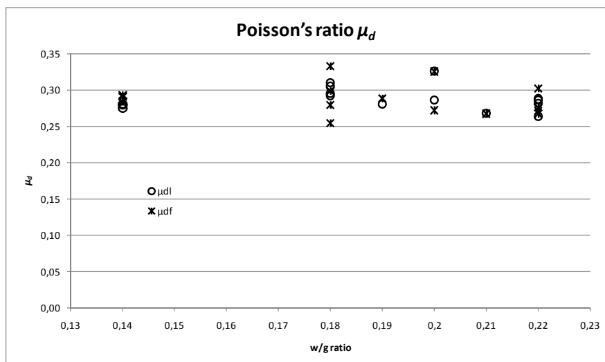
Fig. 6. The Poisson's ratio \mu_d determined based on longitudinal and torsional vibration \mu_{dl} and based on the transversal and torsional vibration \mu_{df}
