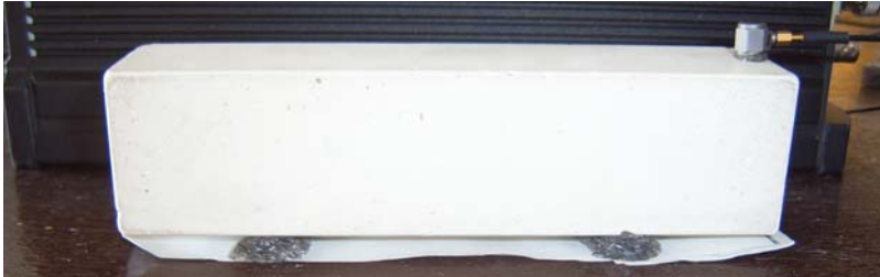
Fig. 2. The impulse excitation method – test arrangement for measurement of fundamental transversal resonant frequency
