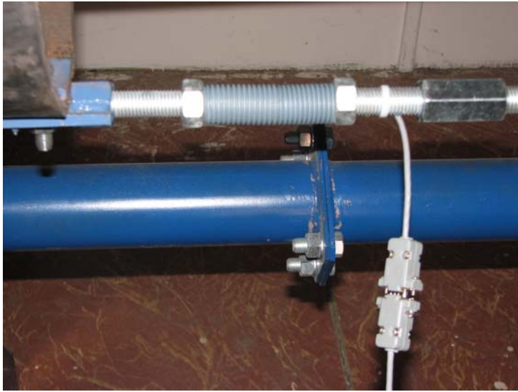
Fig. 4. Tightening screw rod with glued strain-gauges
