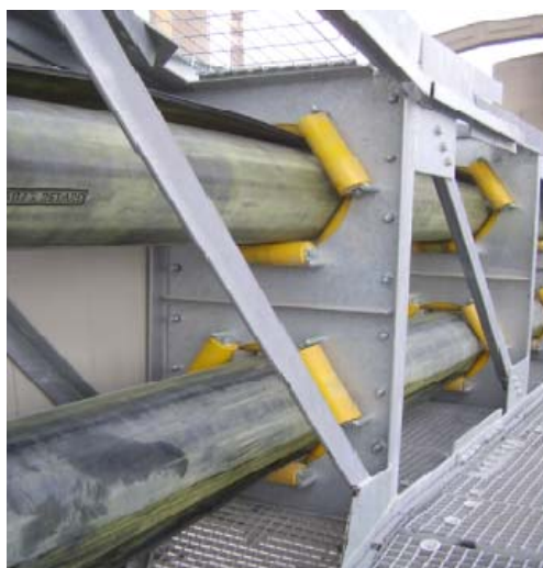
Fig. 1. Upper and lower branch of a pipe conveyor
