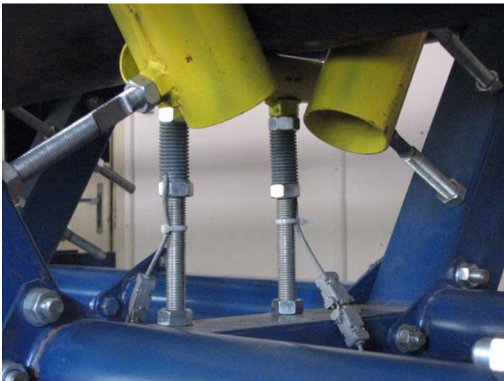
Fig. 3. Substitute of a roller and holders with strain-gauges
