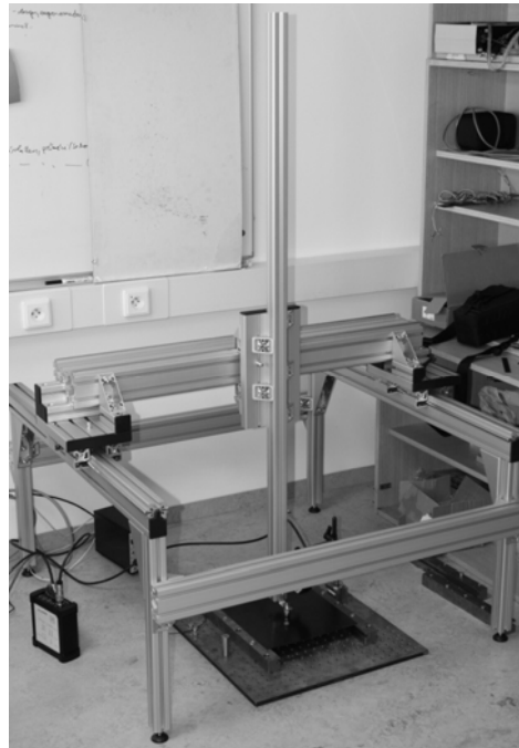
Fig. 6. Drop tester with the laser sensor and the steel stand
