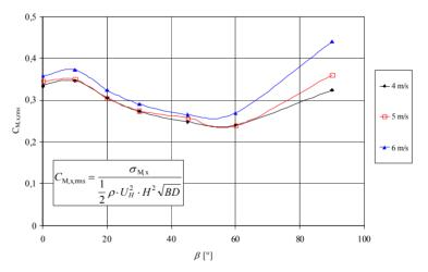
Fig. 6. Measured values of the moment coefficient on the building
