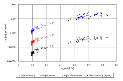
Fig. 4. Dependence of efficient value of the response fluctuation value on the mean value of the wind pressure on the top of the building
