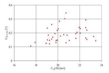
Fig. 5. Measured values of the moment coefficient on the building  $C_{M,x,rms}$
