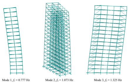
Fig. 3. The lowest natural frequencies and mode shapes of the building
